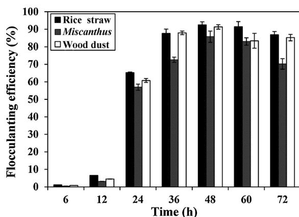
**Fig. 4.** Bioflocs' production along with time by *Pseudomonas* sp. HP2 using 0.5% untreated rice straw, *Miscanthus* and wood dust biomass as carbon source. Values represent mean  $\pm$  SDs ( $n = 3$ ).
