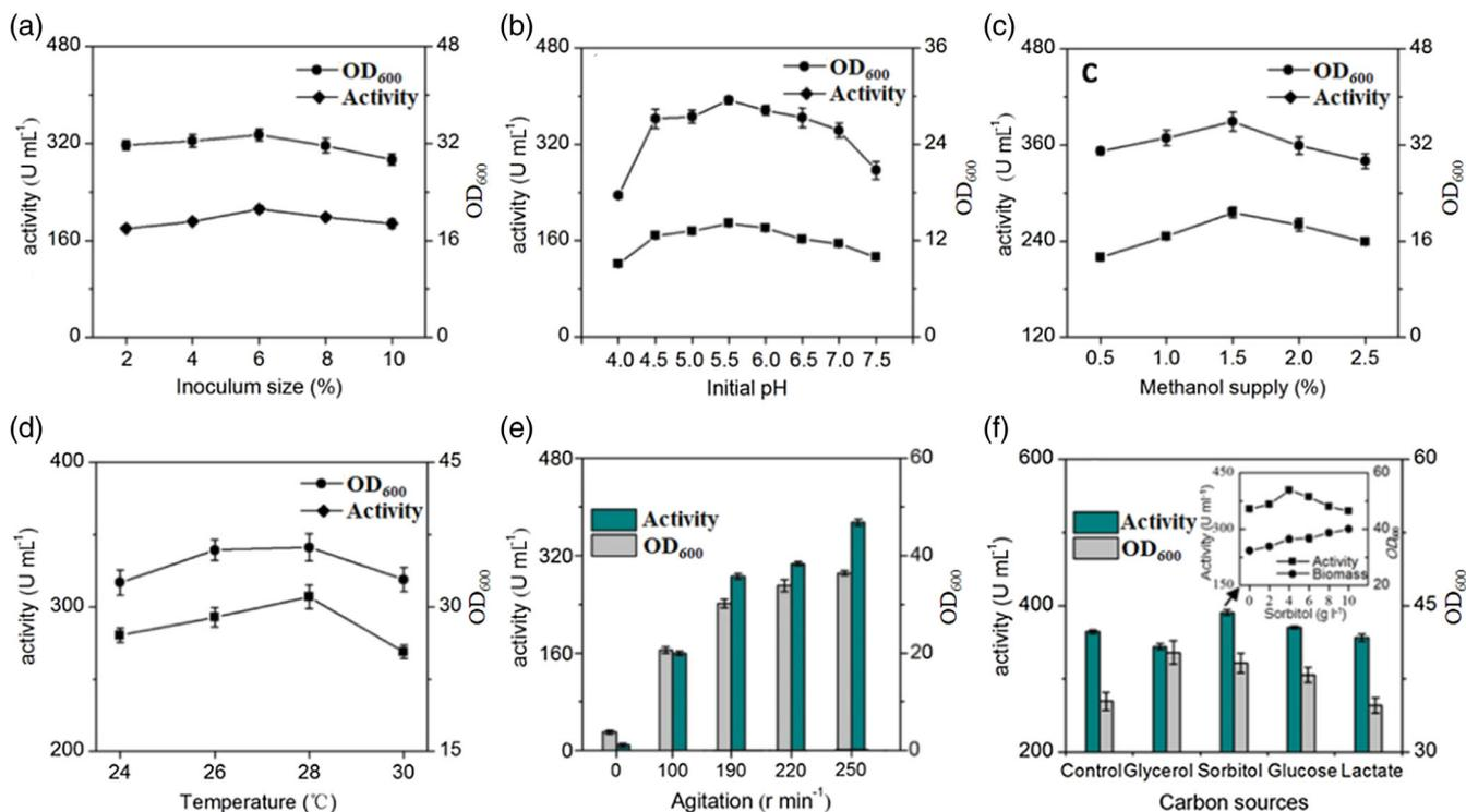
**Figure 4.** The effects of different cultivation conditions on xylanase activity and cell growth at the flask scale: (a) inoculum size, (b) initial pH, (c) methanol dosage, (d) reaction temperature, (e) agitation rate and (f) C sources. Control, cultivation of the double-plasmid transformant without additional C sources. Each value represents the mean of triplicate determinations.
