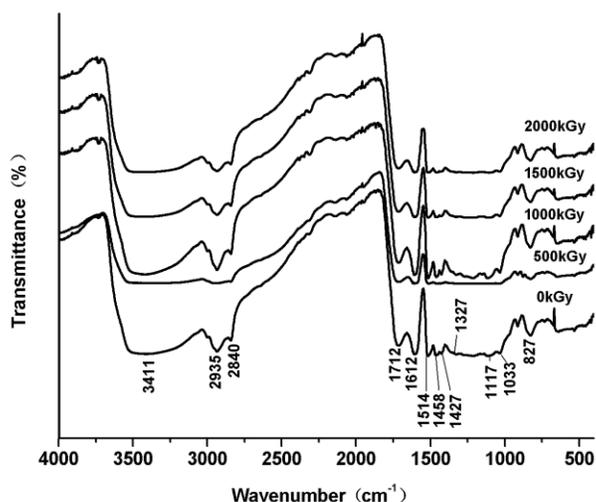
Fig. 5. FTIR spectra of the lignin modified with different doses of irradiation
