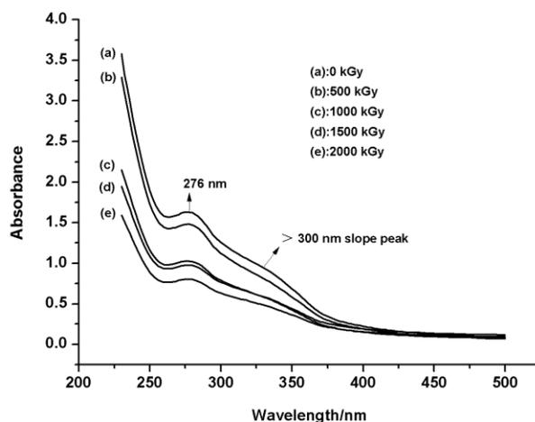
Fig. 4. UV spectra of the lignin modified with different doses of irradiation
