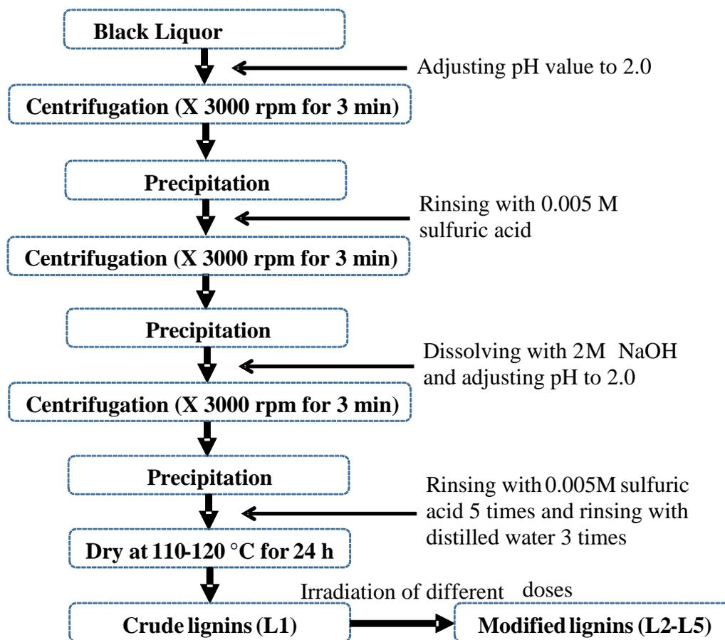
**Fig. 1.** Flow chart showing the extraction and irradiation modification of the lignin
