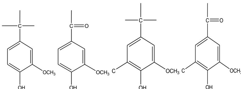
**Fig. 2.** Phenolic hydroxyl groups with different structural characteristics in lignin molecules
