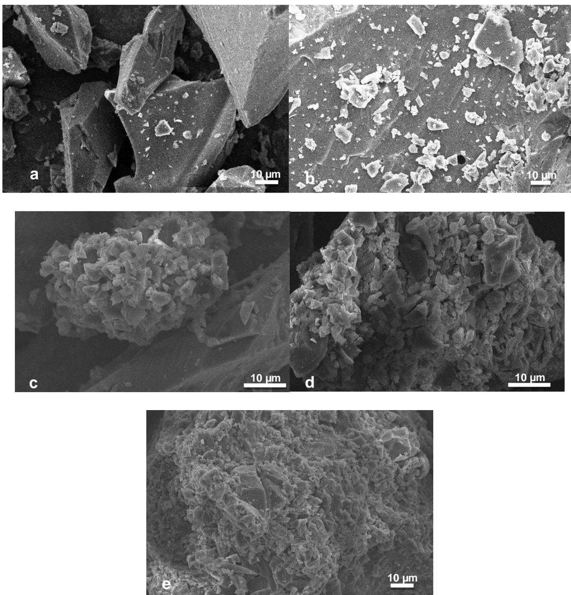
**Fig. 3.** SEM micrographs of the surface morphologies of the crude and irradiation-modified lignins. (a) 0 kGY, (b) 500 kGY, (c) 1000 kGY, (d) 1500 kGY, and (e) 2000 kGY
